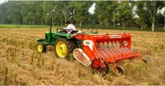
• After harvesting the paddy field using a combined harvester fitted with Super-SMS (Straw Management System) equipment, which chops and evenly spreads the stubble in the field, farmers can directly sow wheat seeds using Happy Seeder with the stubble's organic value adding to the soil.
